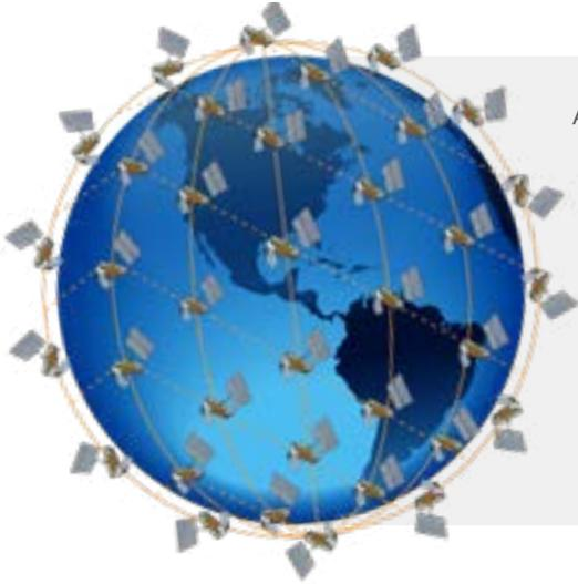
Aireon's space-based, global surveillance system is Automatic Dependent Surveillance-Broadcast (ADS-B) on a satellite. Instead of utilizing traditional radio towers on the ground, Aireon has redesigned them into flexible and highly-effective, space-grade receivers hosted on the global satellite constellation, Iridium NEXT. This allows for 100 percent air traffic surveillance using the same ADS-B avionics already installed on aircraft.
