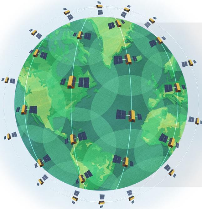
Aireon's space-based, global surveillance system is Automatic Dependent Surveillance-Broadcast (ADS-B) on a satellite. Instead of utilizing traditional radio towers on the ground, Aireon has redesigned them into flexible and highly-effective, space-grade receivers hosted on the global satellite constellation, Iridium NEXT. This will allow for 100 percent air traffic surveillance using the same ADS-B avionics already installed on aircraft.
