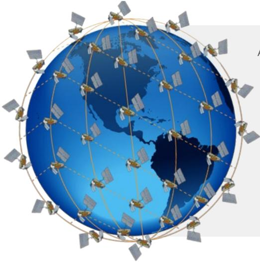
Aireon's space-based, global surveillance system is Automatic Dependent Surveillance-Broadcast (ADS-B) on a satellite. Instead of utilizing traditional radio towers on the ground, Aireon has redesigned them into flexible and highly-effective, space-grade receivers hosted on the global satellite constellation, Iridium NEXT. This will allow for 100 percent air traffic surveillance using the same ADS-B avionics already installed on aircraft.
